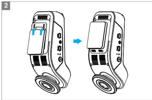
2. Slide the mount horizontally into the slot on the back of the camera.
