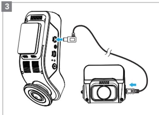
3. Rear camera connection. Power off the product and connect the rear camera cable to the front camera (main unit).
