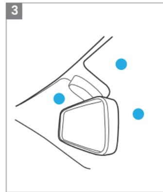
3. Select a location on the windshield behind the rear-view mirror and clean the place. The interior camera must install above the car rear view mirror.
