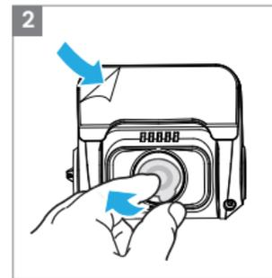
2. Peel the protection film of the sticky pad and camera lens. Fix the rear camera on selected location and adjust lens.
