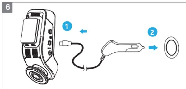
6. Plug the USB power adapter into your vehicle's 12V / 24V female power socket. Insert the long USB cable's male port into the camera's mount USB port.
