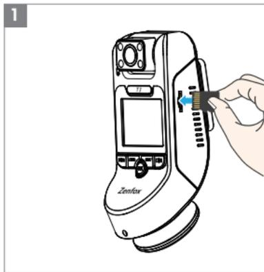
1. Insert microSD card to the slot of the device.
