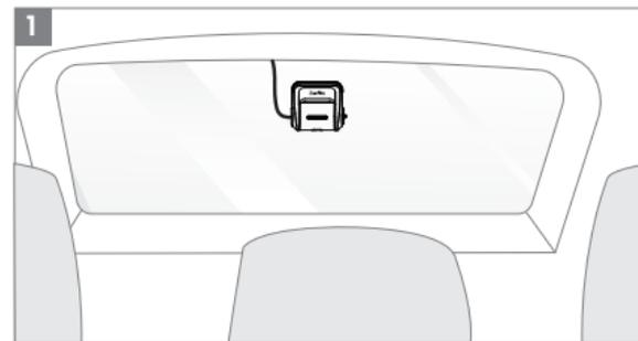
1. Select a location on the windscreen where the camera can record the entire rear view without defrosting grid wires and clean the place.
